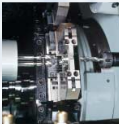
Simultaneous machining from two sides
