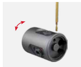
Station 6V, Werkzeug 2, Revolver Querbohren
