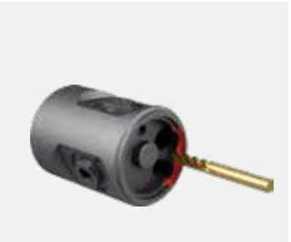
Station 6H, tool 1, turret Milling the recess
