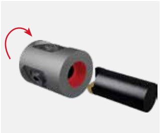
Station 9H, tool 2, turret Core drilling
