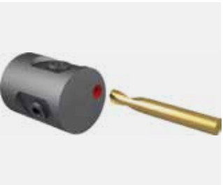
Station 2H, tool 1, turret Rough drilling
