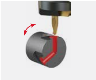
Station 2V, tool 2, turret Cross drilling
