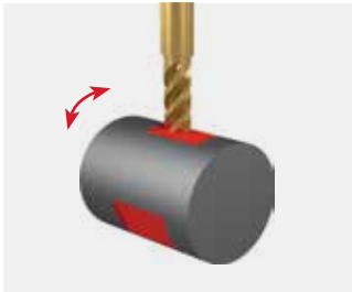
Station 2V, tool 1, turret Milling the surfaces
