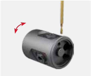
Station 6V, tool 2, turret Cross drilling
