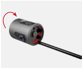
Station 7H, tool 1, Capto holder Internal turning
