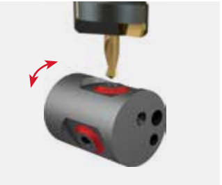
Station 4V, tool 1, turret Slot turning
