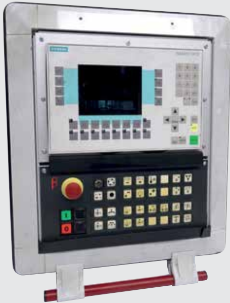
OP27 with an old machine control panel
